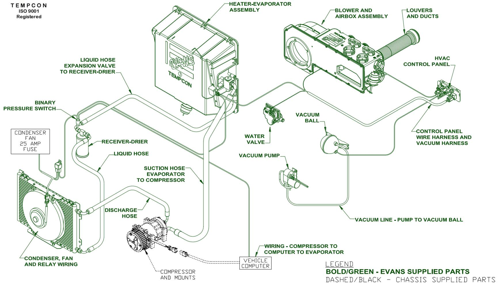
Note: On Workhorse Pusher there is a high pressure switch mounted at the compressor supplied with chassis.
