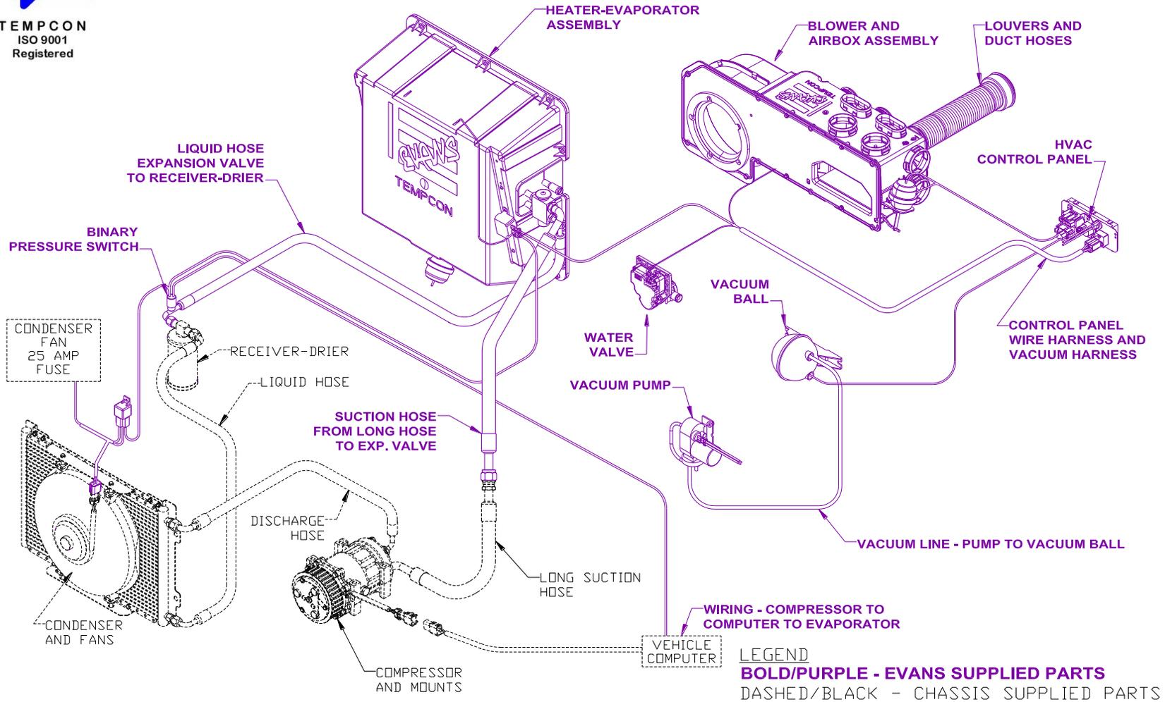
NOTE: On Freightliner and Spartan side radiator/condensers, the pressure switch on the discharge hose that controls the hydraulic fan is chassis supplied. Chassis computer must be enabled to use this switch. There is no Evans supplied electric fan. On Workhorse Pusher there is a high pressure switch at the compressor supplied with chassis.
